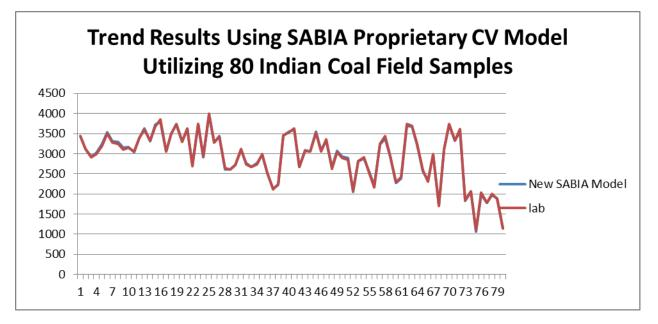
The work with the USGS data base of Indian coal confirmed both that a measurement approach utilizing a carbon reading from the analyzer could work and also that a model significantly better than the Petite Dulong equation would work with the SABIA analyzer. Next it was important to explore actual SABIA site data to confirm the effectiveness of the model.
