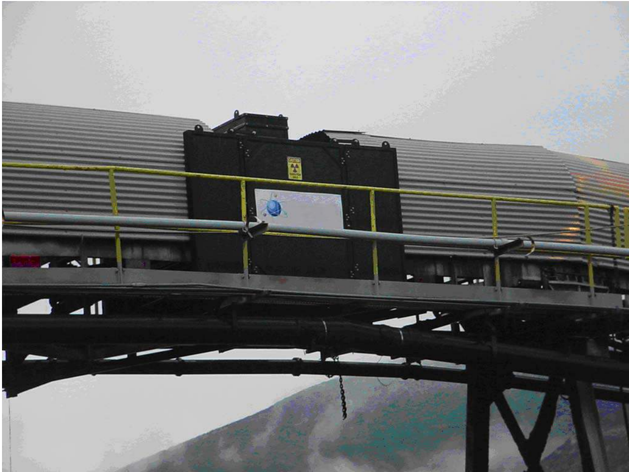
Figure 2. A Version of the technology designed to mount on existing conveyor structure
