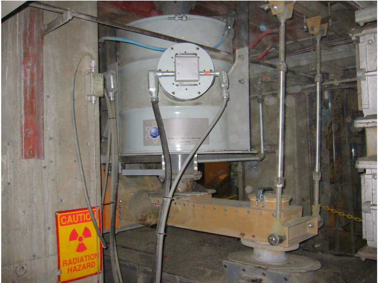
Figure 8. A New PGNA Application – Analyzing Partially Cooled Clinker
