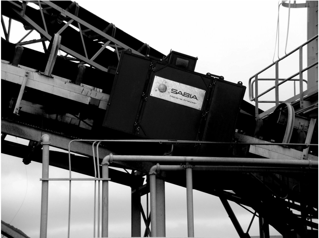
Figure 8. PGNA Analyzer is located on C5A near sampler
