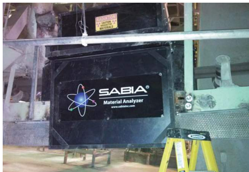
Figure 6 (below): due to the modular nature of the LiNX design, the analyser can fit in a tight space
