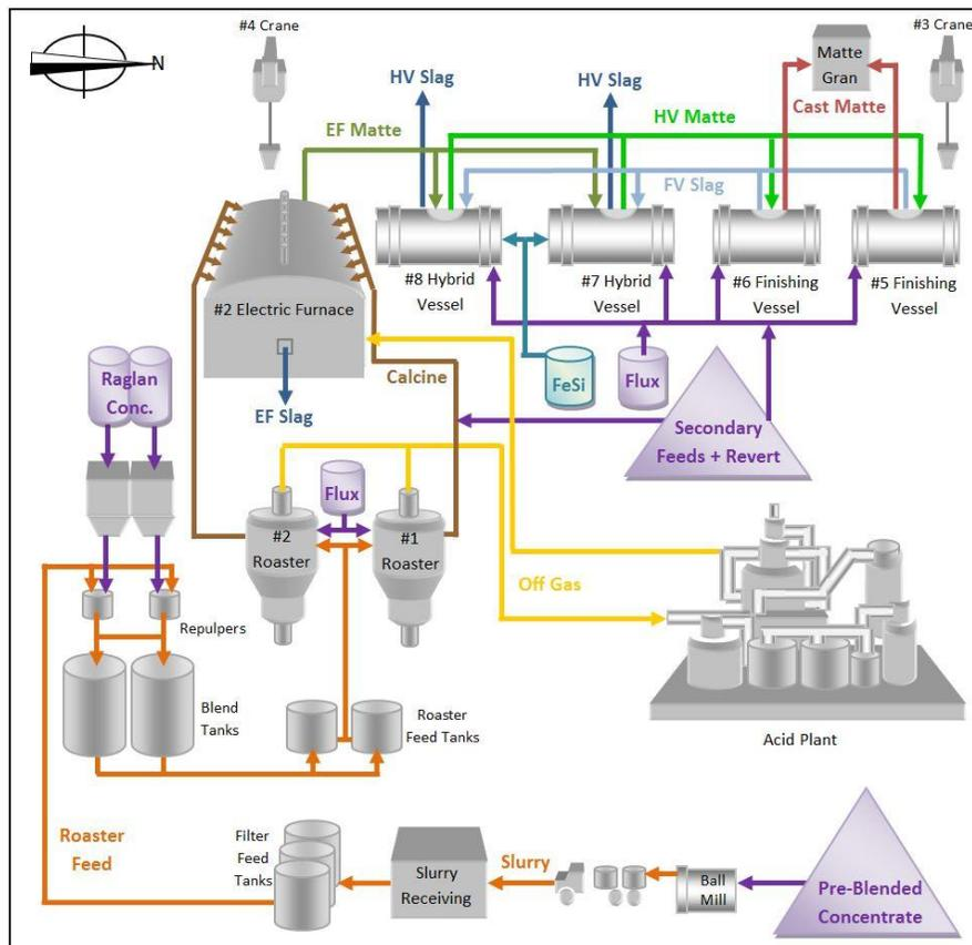
Figure 4 – The Glencore Sudbury Smelter Process
