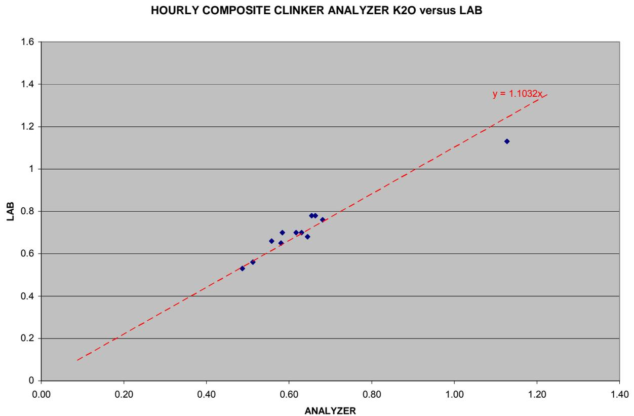
One disappointment in the project has been the inconvenience of dynamic calibrations. The long-term goal of this project would be to input the information into the plant kiln-control software to improve kiln stability and the consistency of the clinker product.
