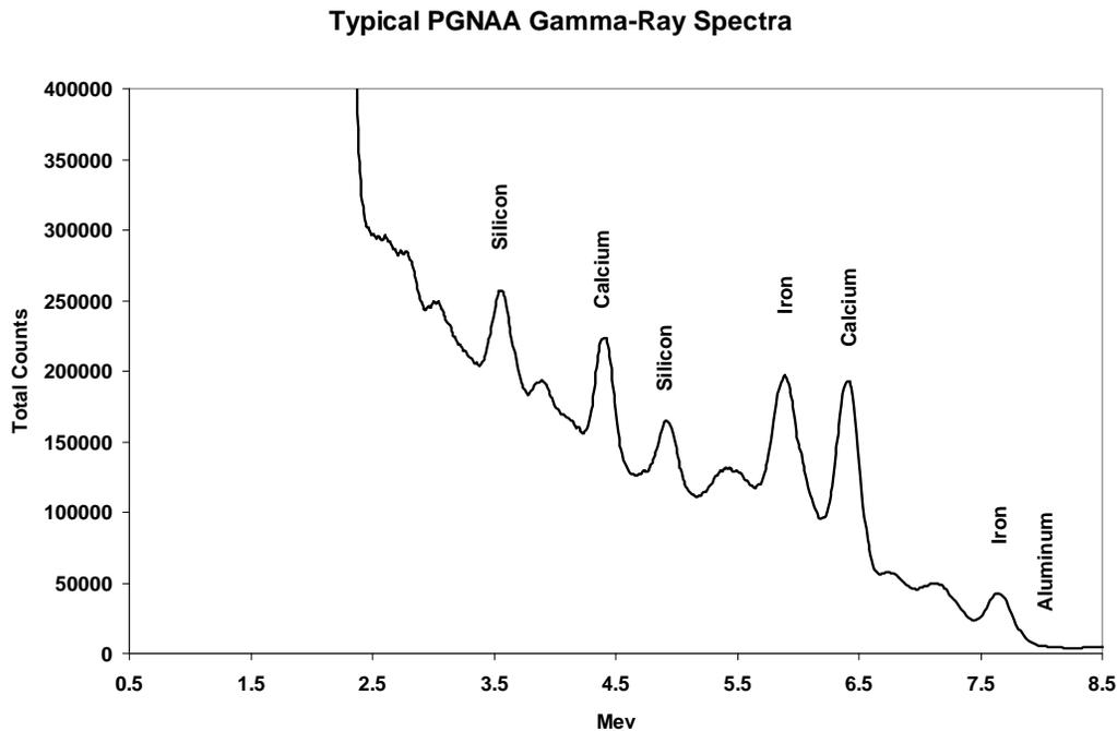
Figure 4. A Typical Gamma Ray High Energy Spectrum
