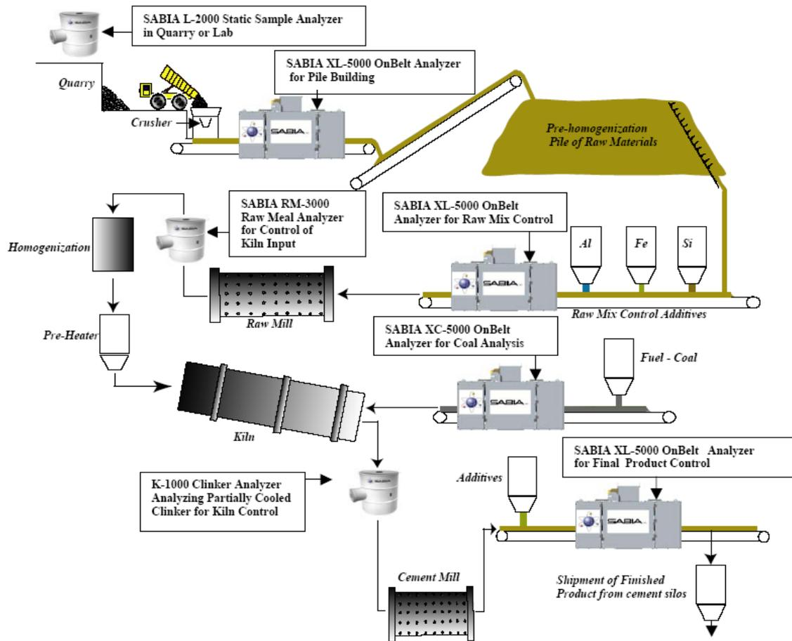
Figure 1. Potential PGNAA applications at a cement plant
